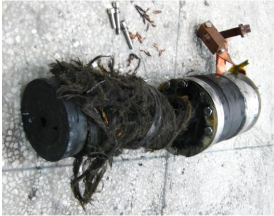
Fig. 3. Photograph of the magnet after failure. The whole magnet winding has been pushed out from the SSS. The G10 flange at the bottom of the magnet was torn into pieces by the magnet winding and several bolts broke.
